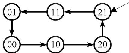
**Figure 5:** Example of a path of the STS of Fig. 2 verifying  $(x = 2) \wedge GF(x = 2)$  (if  $(2, 0)$  or  $(2, 1)$  is the initial state of the path), compatible with  $\mathcal{C}$  but not with  $\mathcal{C}'$ .
