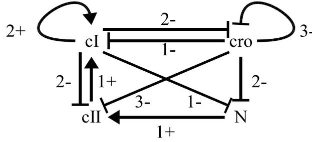
**Figure 6:** Graph of interactions associated with immunity control in bacteriophage lambda. Arrows are labeled by the threshold and sign of the corresponding interaction. For clarity blunt arrows indicate the negative interactions.
