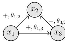
**Figure 1:** The toy network developed for this overview. In all examples we consider that  $\theta_{1,2} > \theta_{1,3}$ , that is,  $x_3$  is transcribed before  $x_2$ . However, we wish to enforce behavior such that  $x_2$  is present before the inhibiting effects of  $x_3$  can take effect.
