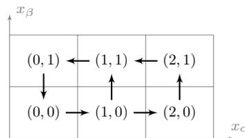
**Figure 2:** A state transition graph of the interaction graph in Figure 1
