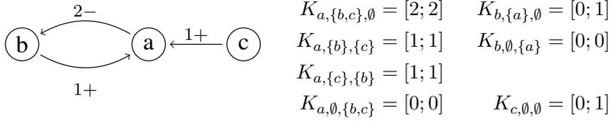
**Figure 2:** (left) IG example. Regulations are represented by the edges labeled with their sign and threshold. For instance, the edge from  $b$  to  $a$  is labeled “1+”, which stands for:  $b \xrightarrow{1} a \in E_+$ . (right) One admissible parametrization of the left IG.
